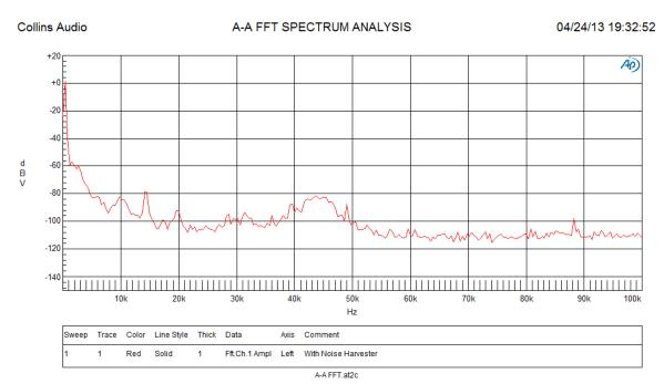
Figure 4. 100kHz FFT With Noise Harvester™
