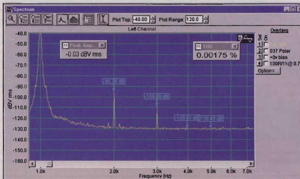
Figure 5: Both second and third harmonics have increased relative to the 0.4 volt test signal. The second much more than the third. Intermodulation components remain buried in the noise floor.
