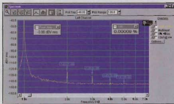
Figure 5: Distortion measurement of a Class 1 ceramic using 100Hz and 1kHz signals at 4 volts and 18 volt DC bias. With no bias this tiny 10nF 50 volt C0G multilayer capacitor measured just 0.00006%. Second harmonic was -128.5dB, the other levels remained as shown.
